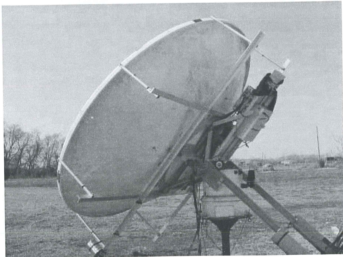
Figure 5. Back structure for 3 Meter Dish at W5LUA
